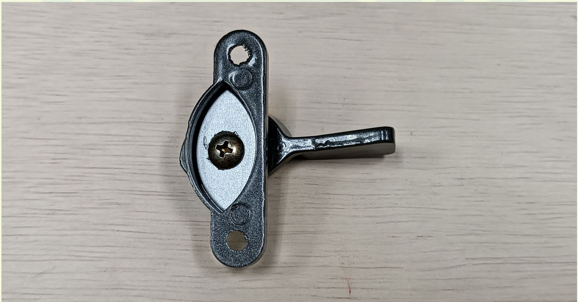
Figure 3: Test samples of DEKKO 005 Crescent Lock (R/L) - Bottom
